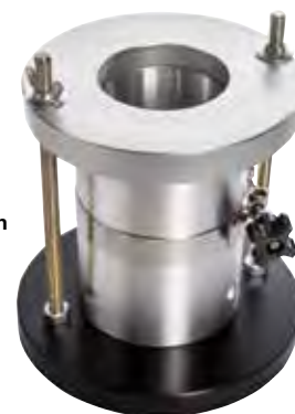
Two-Part Compaction Mold Assembly
