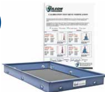
GV-66 Calibration Verification shown with Screen Tray
