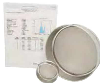
Precision Electroformed Sieves
