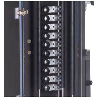
Close-Up of SS-22 Tapping Hammers
