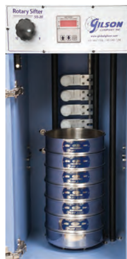
SS-20 inside view shown with 8in Sieves
