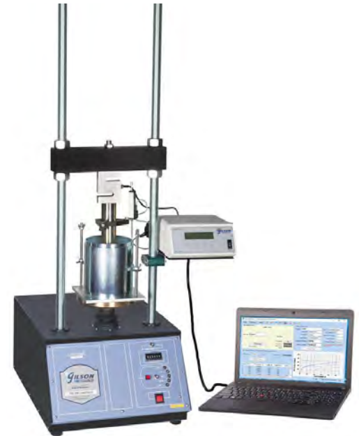
Typical CBR/LBR Test Set-up
