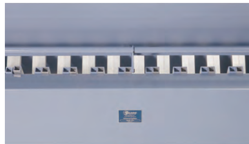
SP-0 close-up of Universal Splitter Chutes
