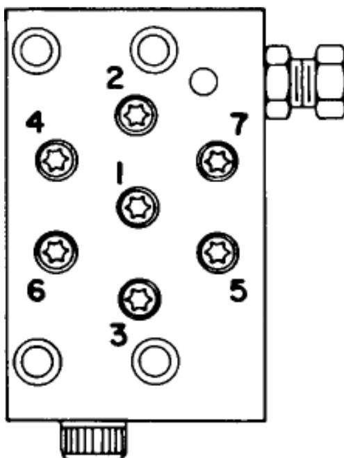
**NOTE:** Assemble in sequence shown. Lubricate under head and on threads. Torque to 170 in. lbs.
