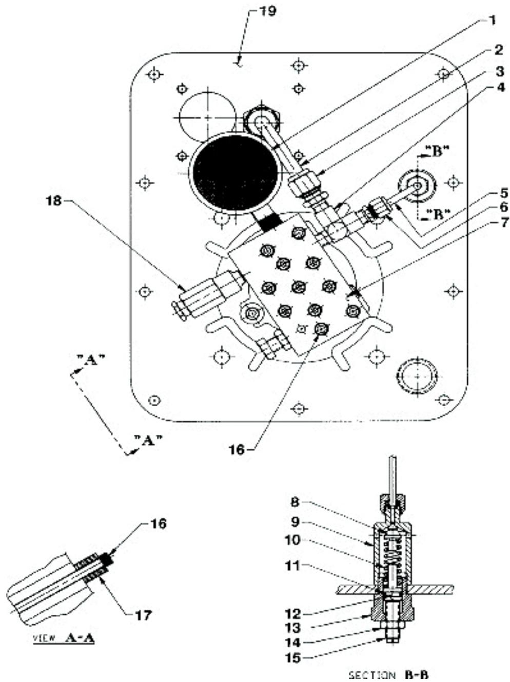
**8.5.2 Parts List and Bolt Tightening Sequence**
