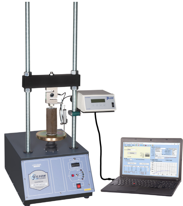
Figure 1: Typical unconfined compression test setup
