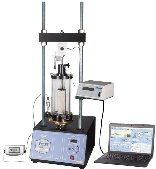
Figure 1: Typical triaxial test setup.
