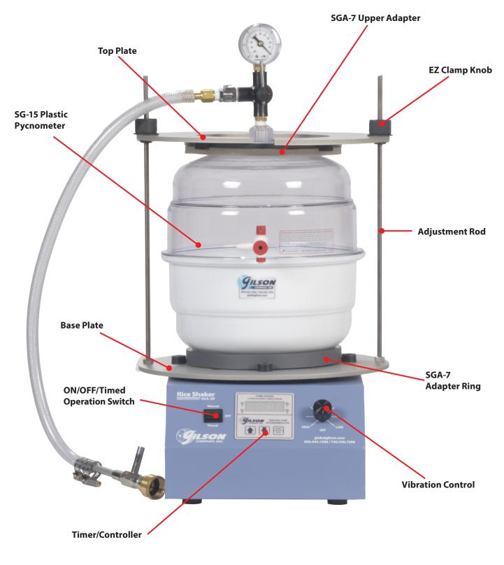
Figure 3 Using SG-15 Plastic Pycnometer
