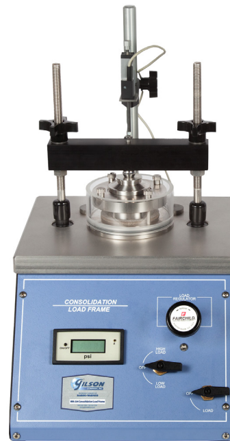
HM-354 shown with floating ring consolidometer and LVDI
