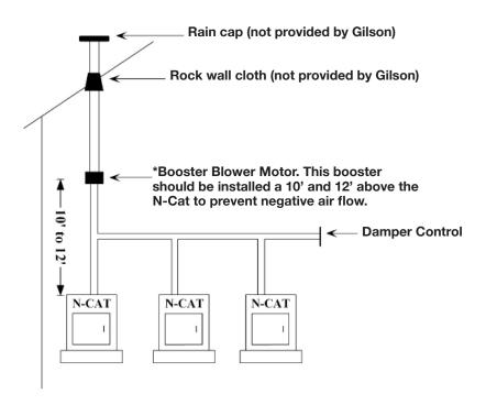
\*Booster Blower Motor should have an ON/OFF toggle switch wired next to the N-Cat main control panel. The blower motor should only be activated with the toggle switch when a test is initiated with the N-Cat. Gilson does not offer a Booster Blower Motor. To size an additional booster blower more, please consult an HVAC technician.
