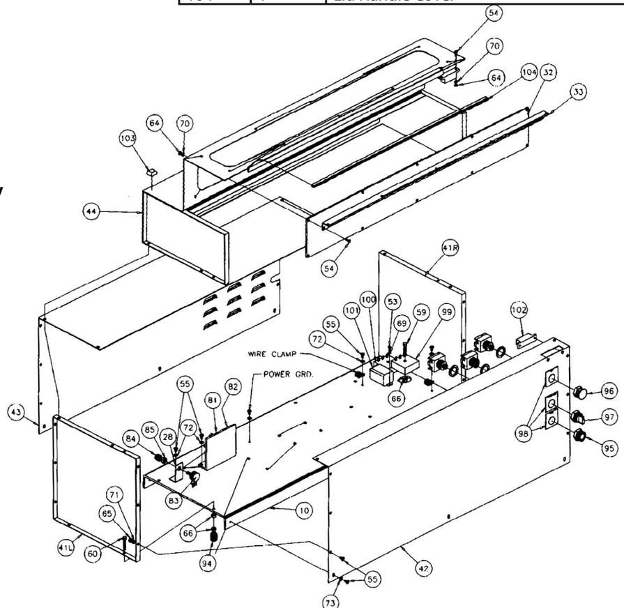
4.2 SE-2B & SE-2BF Base Frame Assembly Parts List & Diagram
