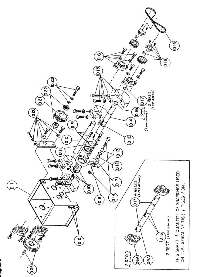
TM-5 & TM-6 Parts Diagram #2 (Drive Assembly)
