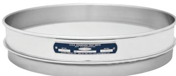
**12in Diameter Stainless Steel Half Height Test Sieve**
