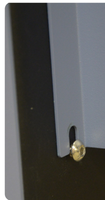
Fig. 10a: Remove bolts for chain adjustment
