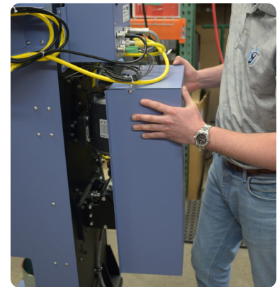
Fig. 10b: Removing cover for chain adjustment
