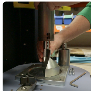
Fig. 3l, 3m: Attaching sector face
