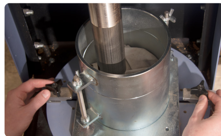
Fig. 6a: Mounting the mold to the machine
