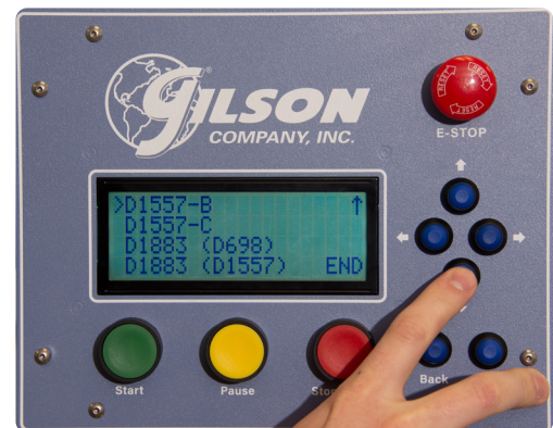
Fig. 7b: HMI / Programmable Digital Controller Arrow Buttons
