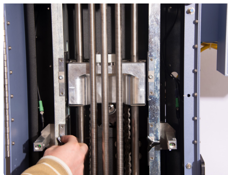
Fig. 4a: Switching the drop height
