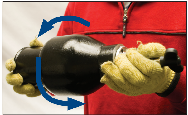
STEP 7B: Using an orbital motion to spin the balls around inside the chamber
