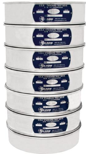
**8in Diameter Stainless Steel Full Height Test Sieves and Pan**
