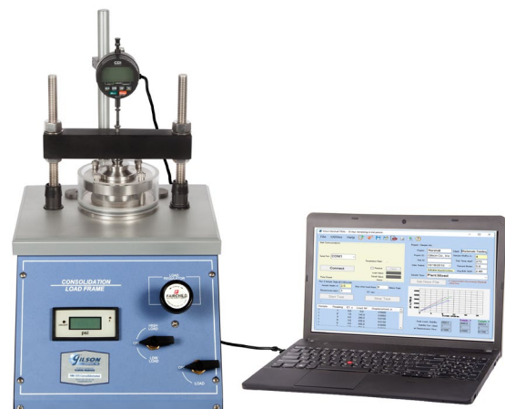
Figure 2: Pneumatic Consolidation Frame with 1in Displacement Transducer and Two-Channel Data Readout Box
