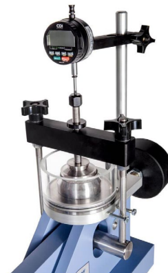
Figure 1: Dead-Weight Consolidation Frame with Digital Dial Indicator
