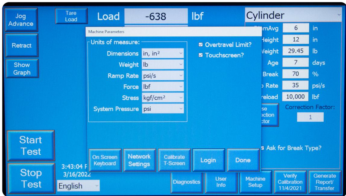
Fig. 6b: Machine Parameters (Machine Setup) Window
