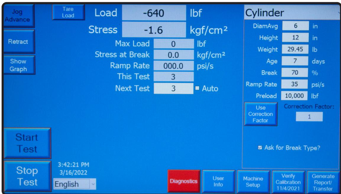
Fig. 6a: HMI (Touchscreen Interface) Buttons on Main Test /Run Screen
