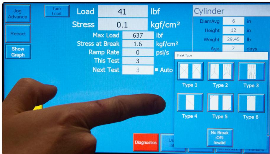
Fig. 6d: Break Type selection window
