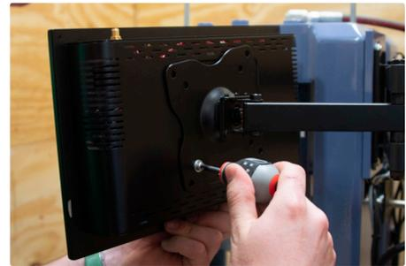
Fig. 2b: Tighten screws—do not overtighten
