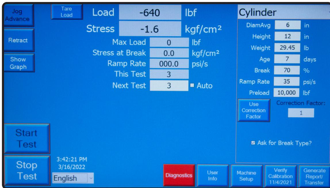
Fig. 6c: Display Fields on Main Test/Run Screen
