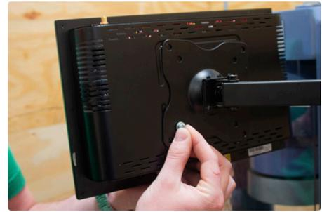
Fig. 2a: Tighten screws with fingers
