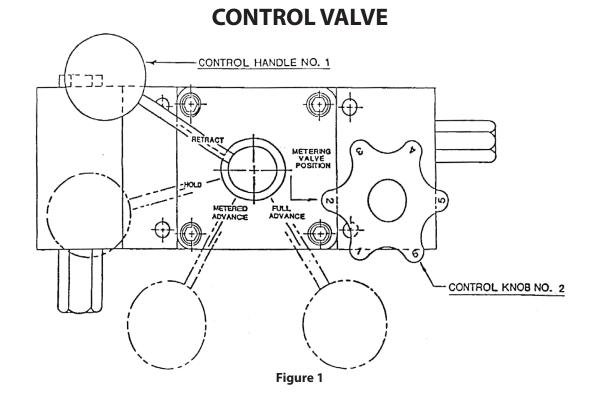
test has been completed, position Valve Control Handle No. 1 to the "retract" position.
