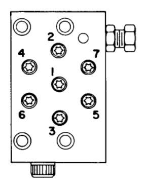
**NOTE:** Assemble in sequence shown. Lubricate under head and on threads. Torque to 170 in. lbs.
