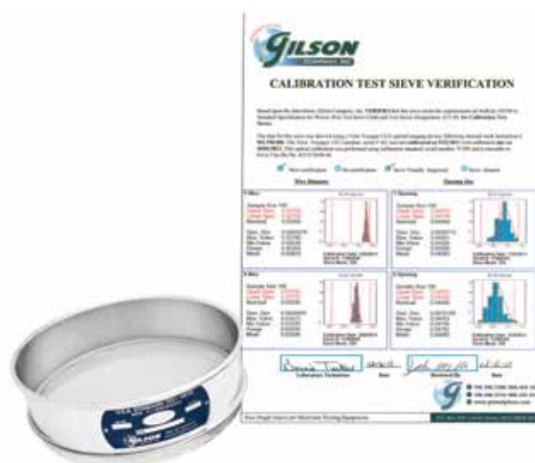
GV-65 Calibration Verification shown with Sieve
