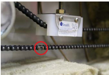
Figure H.7: Disassemble chain master link
