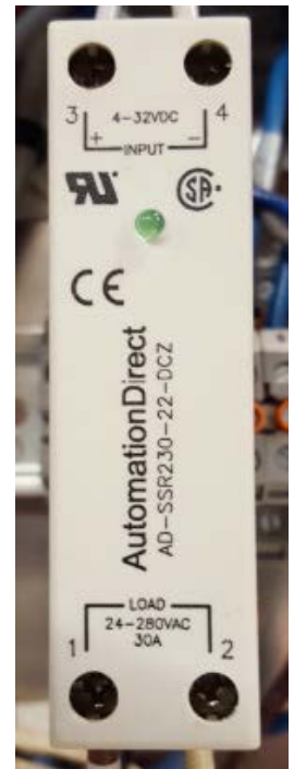
Figure G.5: RTFO heat control
