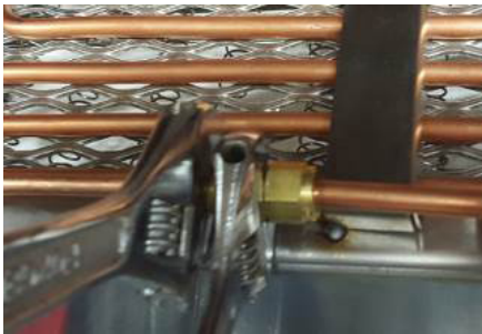
Figure H.1: Disconnect air line coupling
