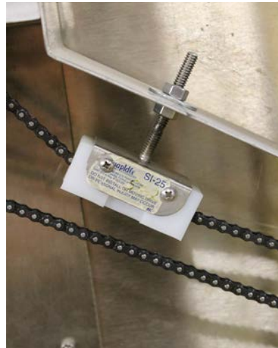
Figure H.10: Chain is properly tensioned
