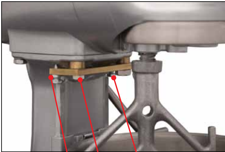
Locking Nuts (2) Motor Mounting Bolts (2) Adjusting Screws (2)
